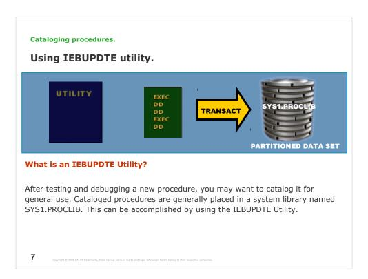
IEBUPDTE is designed to add and replace procedures in a partitioned data set.
