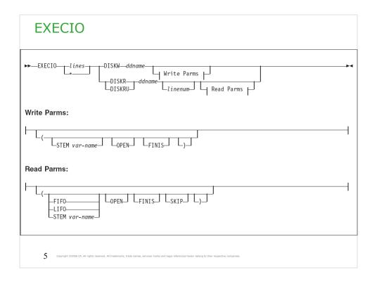
**EXECIO** command controls the input and output of information to and from a data set. Information can be read from a data set to the data stack for serialized processing or to a list of variables for random processing. Information from the data stack or a list of variables can be written to a data set.
